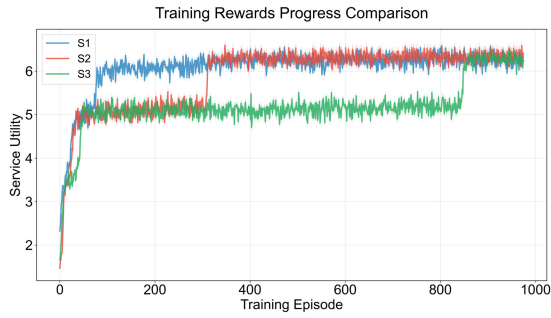
Fig. 3. Convergence of average service utility across three network topologies (S1, S2, S3) over 1M training steps.
