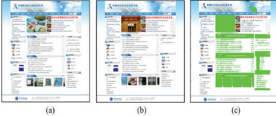
Fig. 7 (a) and (b) are two pages with the same URL; (c) shows the pixels (colored by green) with different colors in (a) and (b).
