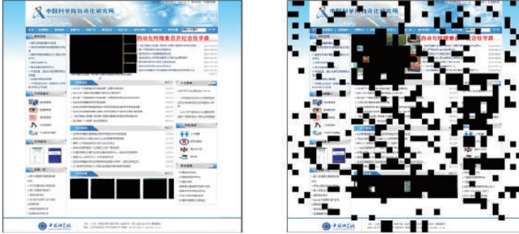
Fig. 5 The benchmark static part of a Web page (left) that was manually determined, and the sampled blocks of the Web page (right) obtained using our method. The black boxes were not included.
