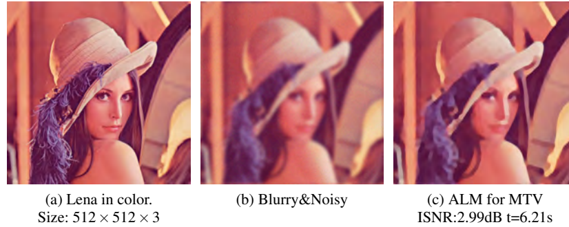
Fig. 7: Augmented Lagrangian method for multichannel TV (MTV) restoration. (b) is a corruption of (a) with within-channel Gaussian blur f_{\text{special}}(' \text{gaussian}', 21, 5) and Gaussian noise with variation 1e-3 ; (c) is the recovered result.
