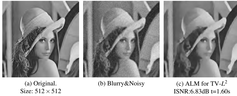
Fig. 3: Augmented Lagrangian method (ALM) for solving TV- L^2 model. (b) is a corruption of (a) with Gaussian blur fspecial('gaussian', 11, 3) and Gaussian noise with variation 1e-2 ; (c) is the recovered result.
