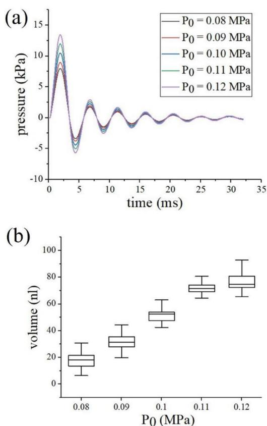
**Figure 4.** (a) Pressure pulse  $P(t)$  in the liquid storage chamber, and (b) droplet volume, for a set of source pressure  $P_0$  at the front-end of the solenoid valve, where  $\Delta t = 1.5$  ms,  $V = 6.46$  kV.
