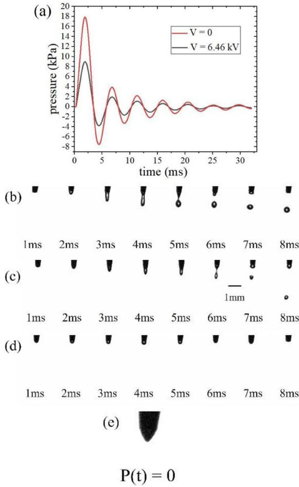
**Figure 2.** (a) Pressure waveforms for producing single droplet per ejection at  $V = 0$  and  $V = 6.46$  kV (b) ejection process for  $V = 0$ , (c) ejection process for  $V = 6.46$  kV. (d) Deformation of the meniscus for the  $P(t)$  shown as black curve in panel (a), and at  $V = 0$ . (e) Meniscus at  $V = 6.46$  kV, without pneumatic actuation.
