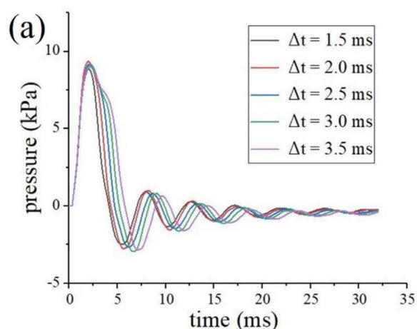
**Figure 5.** (a) Pressure pulse  $P(t)$  in the liquid chamber, and (b) droplet volume, for a set of  $\Delta t$ , where the source pressure is fixed at  $P_0 = 0.09$  MPa,  $V = 6.46$  kV.
