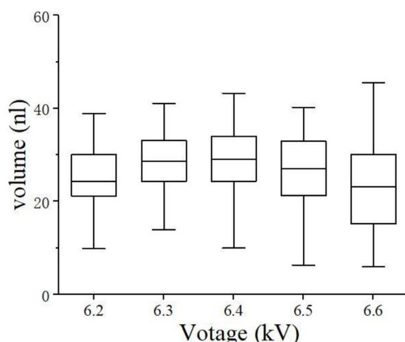
**Figure 6.** Droplet volume ejected under a set of voltage between the nozzle and the collector electrode. The pneumatic actuation is kept unchanged by setting  $P_0 = 0.09$  MPa and  $\Delta t = 1.5$  ms.
