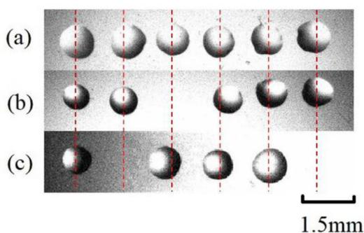
**Figure 3.** Demonstration of the operation mode of DOD ejection. Photograph of micro-droplets sprayed on a glass slide. (a) All ejections are enabled, (b) the third ejection is disabled, (c) the second and sixth ejection are disabled.
