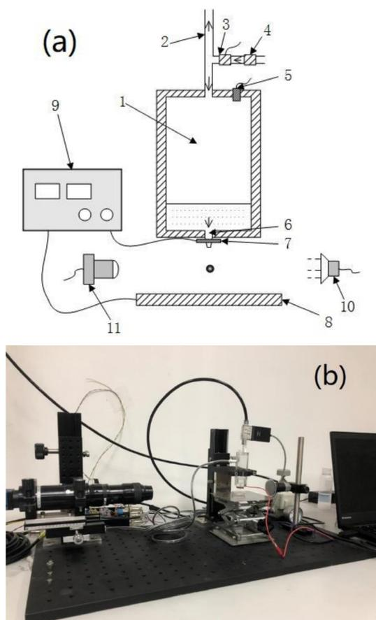
**Figure 1.** (a) Schematic representation of the HPEHD ejection system, where 1 is liquid chamber, 2 is venting tube, 3 is high speed solenoid valve, 4 is pressure regulator, 5 is pressure sensor, 6 is nozzle, 7 and 8 are respective electrodes attached to the nozzle and collector, 9 is high voltage source, 10 is LED illuminator, and 11 is CMOS camera. (b) Real photo of the ejection system.
