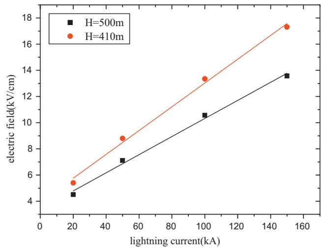
Fig. 7. Relationship between electric field and lightning peak current (neglecting the operation voltage).
