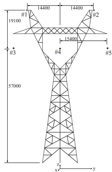
Fig. 4. 1000 kV AC tower (in mm).
