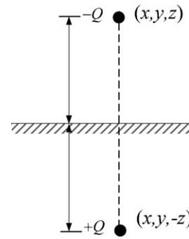
Fig. 2. Image of charge above the ground.
