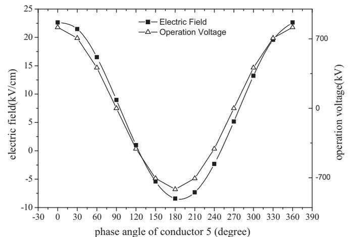
Fig. 11. Surface electric field of conductor #5 with different phase angle.
