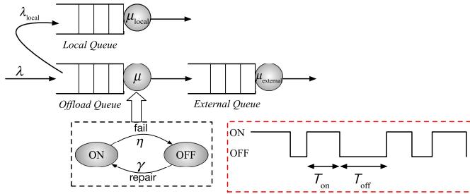
Fig. 2. A queueing model for mobile offloading systems with failures.
