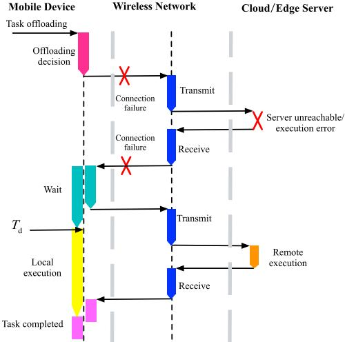
Fig. 1. The delayed offloading model with failures [10].
